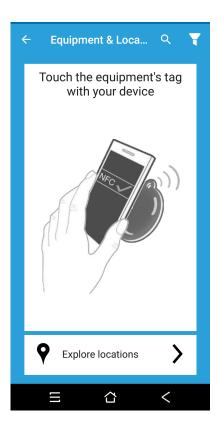
The "Search Equipment & Locations" menu allows you to identify equipment or locations by NFC tag when you touch the tag with your phone (as the next example shows). On the left: the "Equipment Menu" after reading an NFC tag. On the right: the same menu when you scroll down. There are many options to help your daily work, such as the "Technical Sheet", "Registry History" or even "Documents and Photos" that you can add to equipment or locations.
